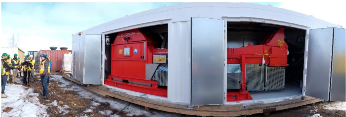
The sensor-based ore sorter that will create a rare earth concentrate delivered to the Nechalacho Rare Earth Demonstration Project in March 2021 over the winter ice road.
